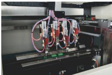
高效率拼版四阀喷涂工艺 High-Efficiency Four-Valve Imposition Coating Process
